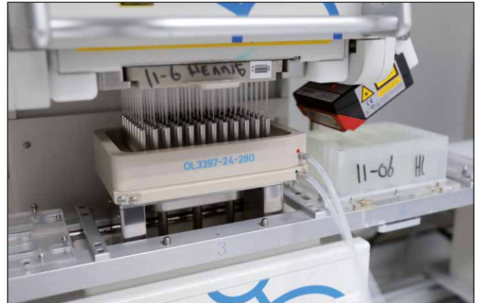
The plates with 96 holes are transferred to a plate with 384 smaller holes.
